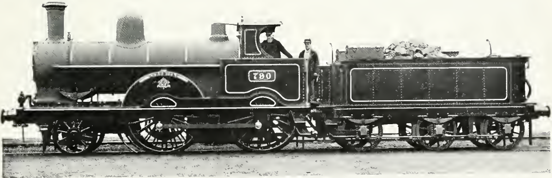
THE "HARDWICKE," which created a record in the "Race to the North" (1895) by running from Crewe to Carlisle—141 miles—at an average speed of 67.2 miles per hour.
