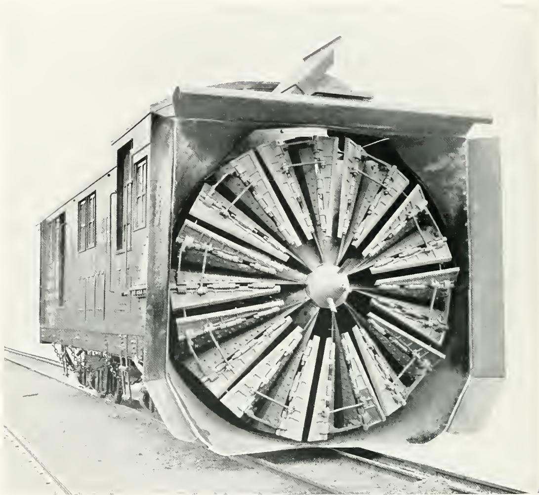
FRONT VIEW OF THE CHICAGO, MILWAUKEE AND PUGET SOUND RAILWAY'S HUGE ROTARY SNOW-PLOUGH.
