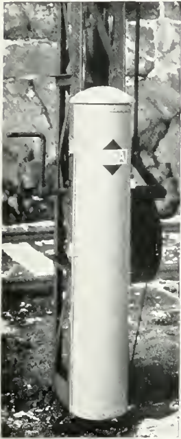
NEW TYPE ACCUMULATOR-BOX OF THE AGA FLASHLIGHT—SHUT.
