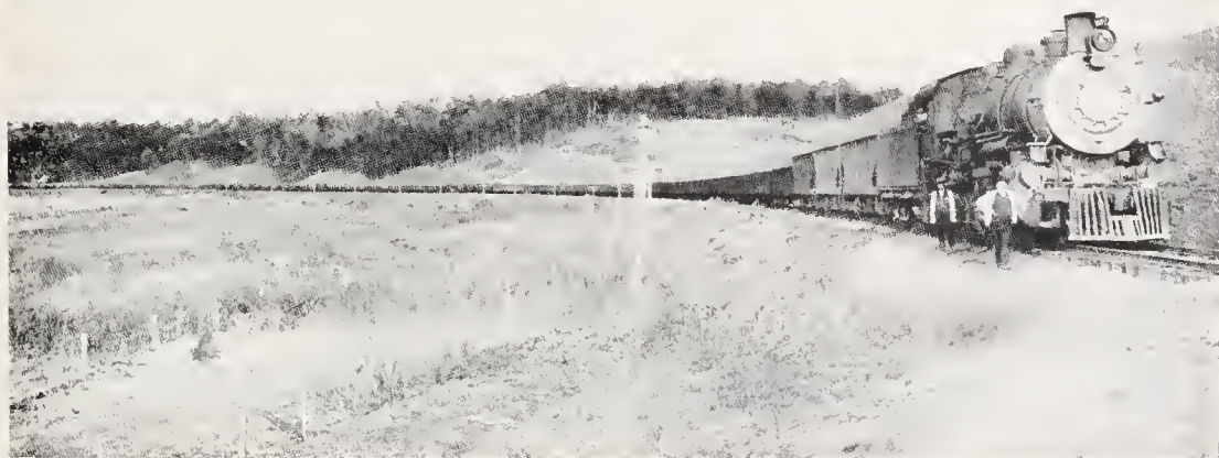
TRAIN OF 80 50-TON LOADED CARS (4,000 U.S. TONS) OF COAL EN ROUTE FROM THE ASSEMBLING YARD AT PRINCETON, WEST VIRGINIA, TO TIDEWATER, SEWALL'S POINT, VIRGINIA.
